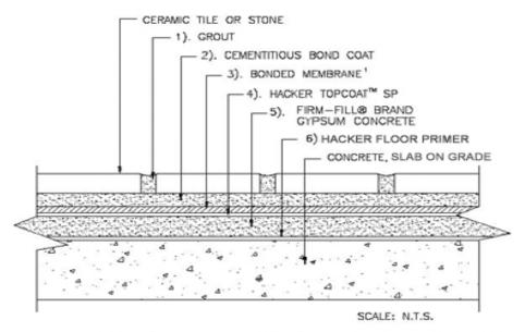
NOTE: BONDED MEMBRANE MAY NOT BE COMPATIBLE WITH HACKER TOPCOAT™ SP.
