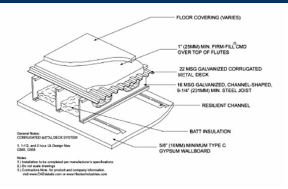
When installed over steel truss, FIRM-FILL® CMD provides an economical lightweight solution for multifamily and mid-rise commercial applications. FIRM-FILL® CMD achieves excellent fire and sound ratings while providing a superior crack-resistant surface for the installation of finished floor coverings.
