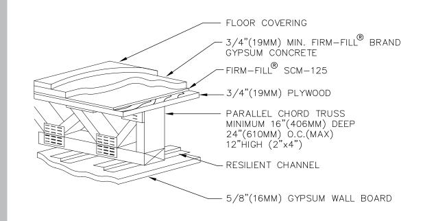
When installed over open web, 0.75" (19mm) FIRM-FILL® Brand Gypsum Concrete and 1/8" (3mm) FIRM-FILL® SCM-125 achieve excellent fire and sound ratings while providing a superior crack-resistant surface for the installation of finished floor coverings.
