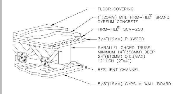
When installed over open web, 1" (25mm) FIRM-FILL® Brand Gypsum Concrete and 1/4" (6mm) FIRM-FILL® SCM-250 achieve excellent fire and sound ratings, while providing a superior crack-resistant surface surface for the installation of finished floor coverings.
