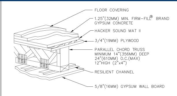
When installed over open web, 1.25" (32mm) FIRM-FILL® Brand Gypsum Concrete and Hacker Sound Mat II achieve excellent fire and sound ratings, while providing a superior crack-resistant surface for the installation of finished floor coverings.
