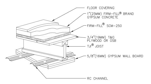
When installed over an I-Joist, 1" (25mm) FIRM-FILL ® Brand Gypsum Concrete and 1/4" (6mm) FIRM-FILL® SCM-250 achieve excellent fire and sound ratings, while providing a superior crack-resistant surface surface for the installation of finished floor coverings. crack-resistant surface for the installation of finished floor coverings.
