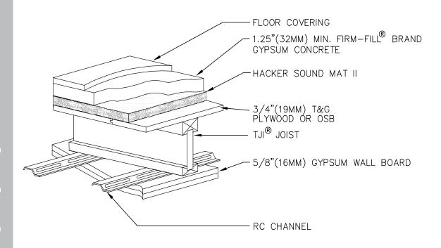
When installed over an I-Joist, 1.25" (32mm) FIRM-FILL® Brand Gypsum Concrete and Hacker Sound Mat II achieve excellent fire and sound ratings, while providing a superior crack-resistant surface for the installation of finished floor coverings.
