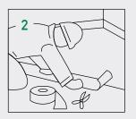
Seams between sound mat rolls are adhered with tape.
