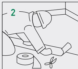
2 Seams between sound mat rolls are adhered with tape.
