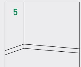
5 Finished floor coverings can be installed when the gypsum concrete is completely dry. Consult flooring contractor for acceptable levels of moisture and recommended procedures for testing dryness.
