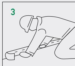
3 Isolation strips are installed, then taped, around the perimeter of the whole room and around any vertical penetrations of the floor.
