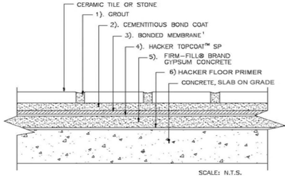
NOTE: <sup>1</sup>BONDED MEMBRANE MAY NOT BE COMPATIBLE WITH HACKER TOPCOAT™ SP. PLEASE CONTACT THE BONDED MEMBRANE MANUFACTURER FOR THEIR RECOMMENDATION.
