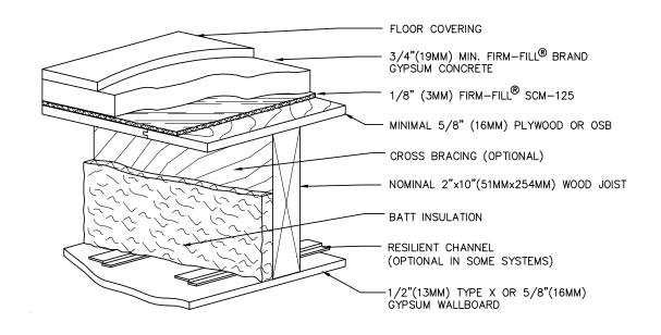
When installed over Nominal Wood Joist, 0.75" (19mm) FIRM-FILL® Brand Gypsum Concrete and 1/8" (3mm) FIRM-FILL® SCM-125 achieve excellent fire and sound ratings, while providing a superior crack-resistant surface surface for the installation of finished floor coverings.
